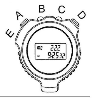
Press button **C** to go into lap mode (the word lap should be visible on the left upper corner of the LCD screen)
